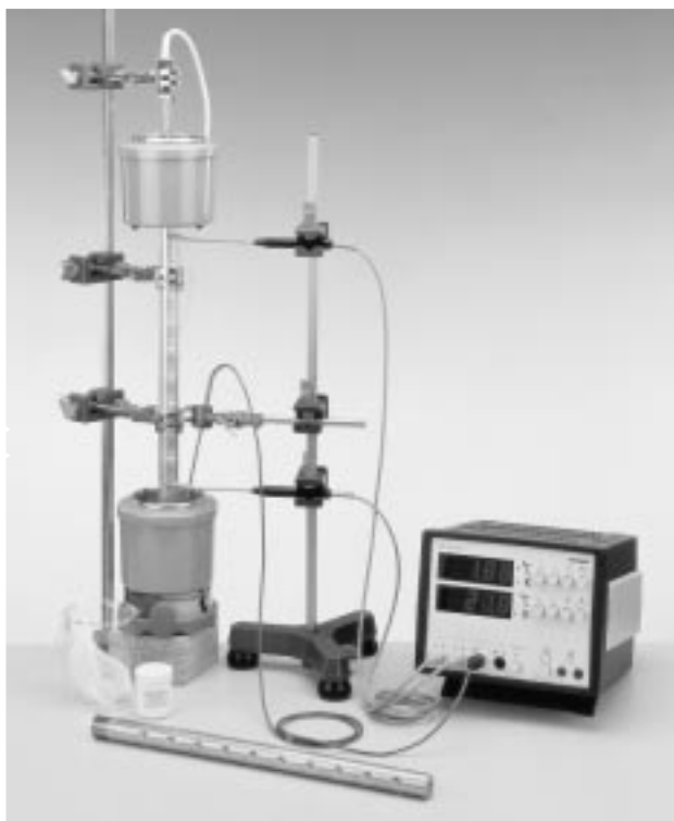
Fig. 2: Complete experimental set-up for the determination of the thermal conductivity of Cu and Al
